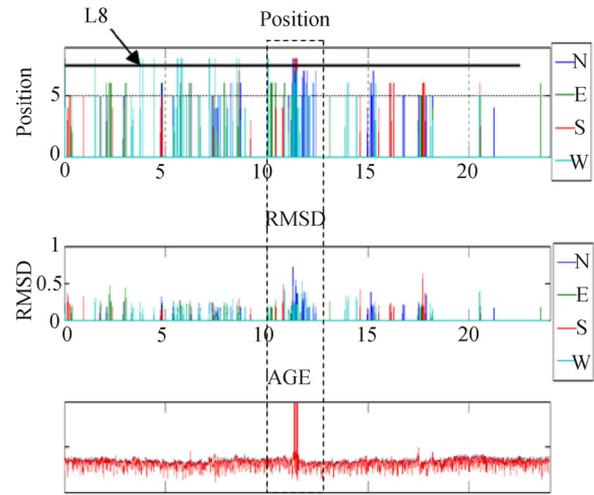
**Fig.4.** Trends for detecting BF channeling (with channeling occurrence).
