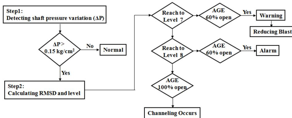
Fig.6. Identification process of BF channeling.
