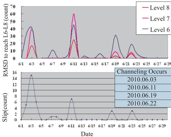
**Fig.3.** Count of RMSD above L6 versus date while comparing with the count of burden slip and time of channeling occurrence.
