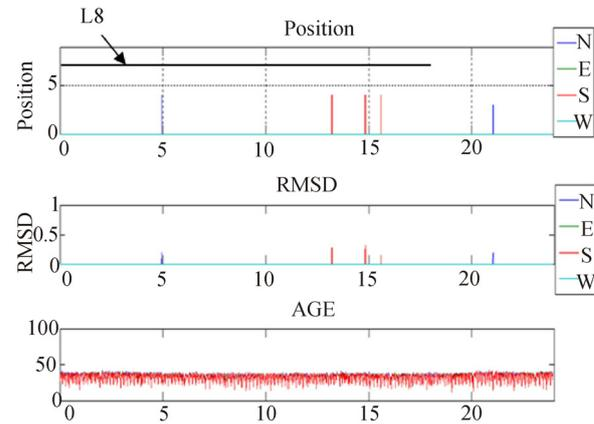
**Fig.5.** Trends for detecting BF channeling (without channeling occurrence).
