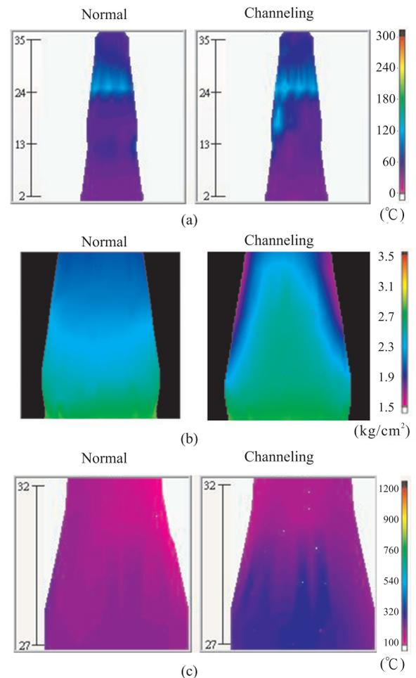
**Fig.2.** Diagram of visual model for the distribution of : (a) shaft temperature; (b) shaft pressure; and (c) skin flow temperature.
