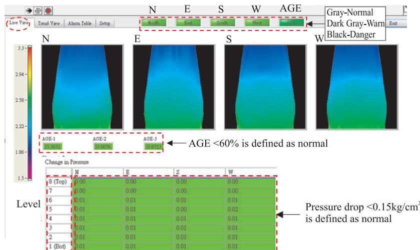
Fig.7. “Live View” for normal BF conditions in this system.
